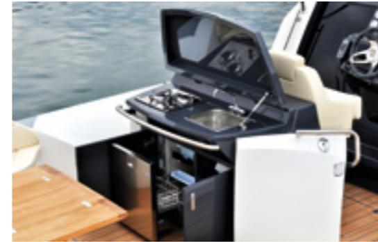
The helm station is ergonomically designed to allow the driver to maneuver in total comfort and safety. The ergonomic seats and the perfect location of controls and instrumentation are the result of a project carefully developed and tested. A kitchenette equipped with sink, hob and refrigerator for snacks or lunches on board
